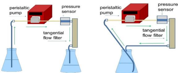
**Figure 1: Experimental setups.** Schematic of single pass experiments (Left). Schematic of close loop paradigm (Right).
