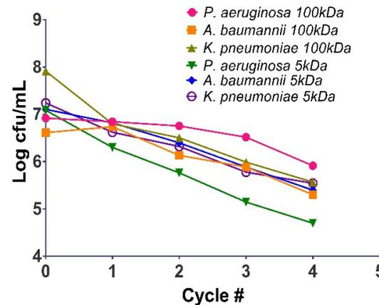
**Figure 5: CFU Reduction.** Using a closed loop system, both 5 kDa and 100 kDa filters were capable of reducing PAK CFUs during a 5 hour time course.
