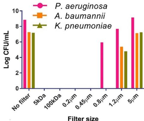
**Figure 2: Size Exclusion.** PAK was passed through TFF and dead-end filter paradigms (single-pass) to evaluate the ability of each to completely eliminate PAK.
