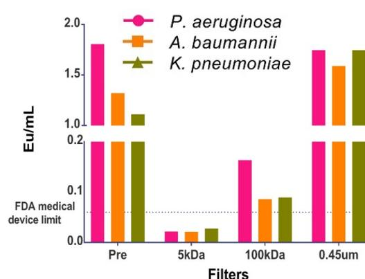
**Figure 3: Endotoxin Filtration.** The LAL assay was used to quantify the reduction of endotoxin after a single pass through 5kDa TFF, 100 kDa TFF, and 0.45 µm dead-end filters.
